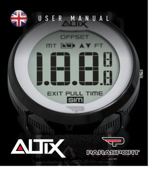
AltiX is a digital altimeter designed to be easy to use and clear to read. Only basic altimeter functions are available, with the addition of a simulation mode, helping training students to recognize the altitude during ground training. It also records exit and pull altitudes, as well as freefall time and average freefall speed, of last jump.
