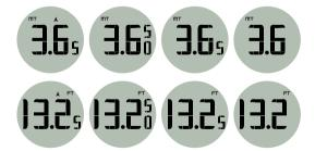
**SIMULATION** - Useful to practice altimeter reading, the function simulates a jump and canopy ride to the ground. Can be interrupted by clicking the button. Exit and pull altitudes can be adjusted (see the respective functions below). Entering the simulation mode, the LCD will briefly show the pull altitude set, and then the exit altitude. Press the button to start the simulation.
