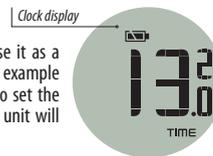
You can also adjust the time by holding the button depressed when the time is shown. Once in clock setting mode you can increase hours first by clicking the button (the up arrow is shown to indicate you're adjusting the hours). Hold key depressed to set minutes (the down arrow is now shown to indicate you're adjusting the minutes). Click to increase minutes, hold key depressed to save the clock setting. Hours are shown in 24 hours format only.
