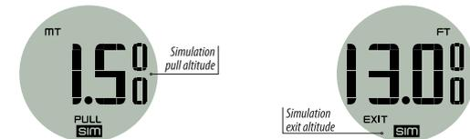
**WARNING - SIMULATION MODE DISABLES ALTIMETER FUNCTION. DO NOT LOAD THE AIRCRAFT WHILE THE SIMULATION IS RUNNING.**
