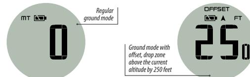
In order to save battery, the unit will go to battery saving mode showing the time. You can show the ground mode by pressing the button. At take off, the unit will automatically switch to altimeter from both clock and ground modes.
