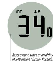
Reset ground when at an altitude of 340 meters (display flashes).
