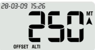
*Ground mode with an offset set as drop zone at +250 m from take off place*
